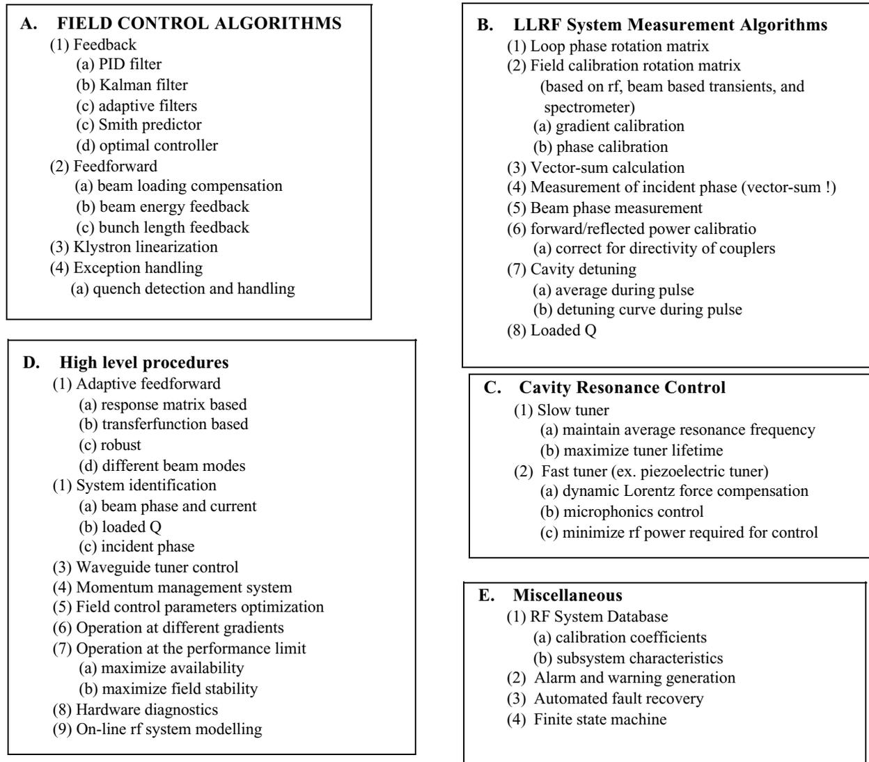
Figure 2: Algorithms and procedures required for an automated digital feedback system.
