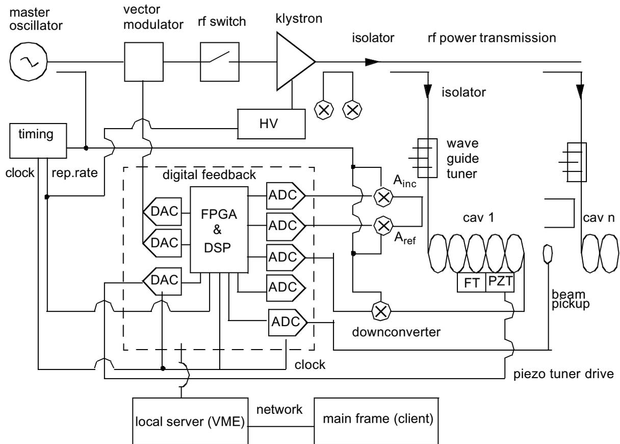
Figure 1: Typical configuration of an RF control system using digital feedback control.
