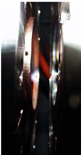
Wake fields excited in a small gap by ampere beams have enough amplitude to heat the vacuum valve. The electric component of these fields can be above the arcing limit. Fig. 3 presents the photo of the disconnected flanges and a gap ring. Traces of breakdowns can be easily distinguished by discolorations on the stainless steel flange at the right side. After replacing the ring with one that has the proper size, the RF heating and the temperature oscillations stopped.
