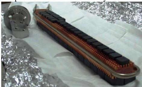
Figure 6: Water-cooled HOM absorber.
