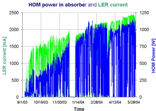
Figure 8: HOM power dissipated in the absorber (blue line) and positron current (green line)
