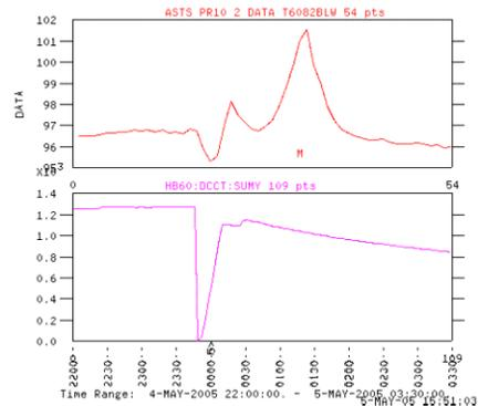
Figure 15: Temperature of the bellows (°F, upper plot) and HER Current (mA, down plot).
