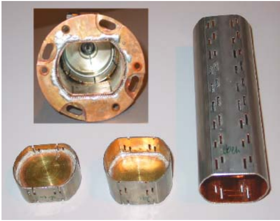
Figure 4: The coax-to-beam-pipe adapter and the three standards for waveguide calibration
