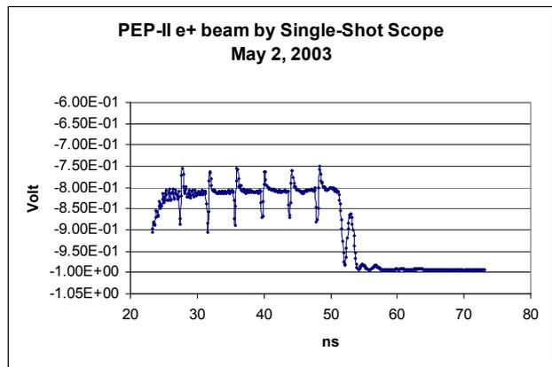
Figure 8: e+ Bunches Captured by the Single-Shot Scope show that multiple bunches can be measured
