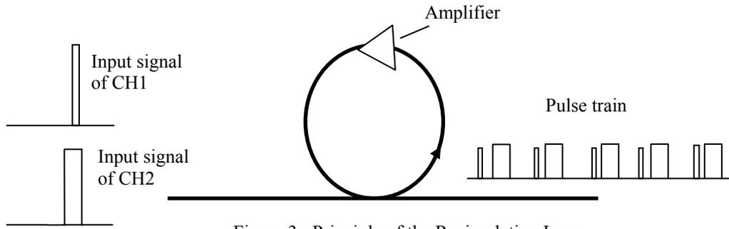
Figure 3: Principle of the Recirculating Loop.
