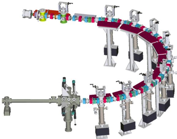
Figure 3: Current experimental setup of 180° of the complete electron ring.
