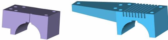
Figure 4: Current magnet mount block (left) and prototype redesign (right).
