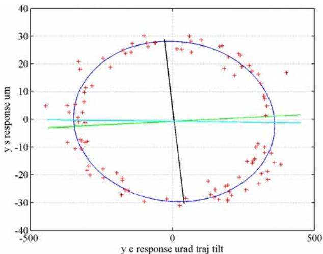
Figure 5: Scaled  $I/Q$  response from the cavity BPM, same data as figure 4. The horizontal scale is in units of trajectory angle (urad) and the vertical scale is in um. The small angle between the plot vertical and the actual vertical  $I/Q$  direction is not corrected.
