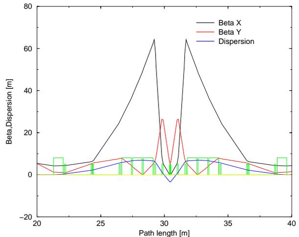
Figure 2: Optics of the stretcher/compressor
