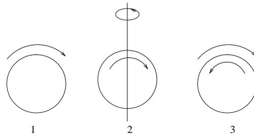
Figure 5: Maintaining beam magnetization across solenoid gaps. Focusing with quadrupole: 1 - the fringe field of the first cooling solenoid creates a vortex. 2 - A quadrupole section rotates the vortex around the vertical axis. 3 - the fringe field of the second cooling solenoid stops the vortex.
