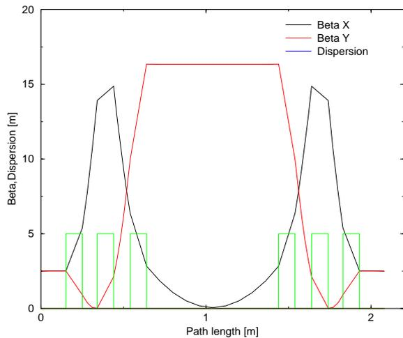
Figure 3: Optics of the matching section between the cooling solenoids
