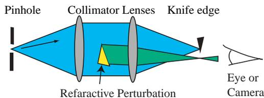
Figure 1. The Schlieren principle
