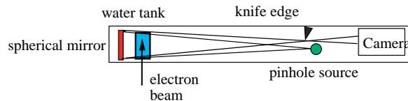
Figure 2, Transverse optical path and beam
