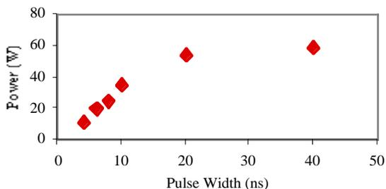
Figure 4, Beam power vs pulse length, at 30 Hz.
