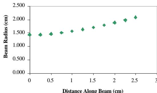
Figure 6, The beam size in the test cell
