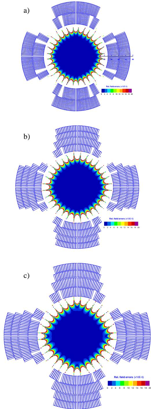
Figure 1: Quadrupole coil cross-sections with 90-mm (a), 100-mm (b) and 110-mm (c) apertures.
