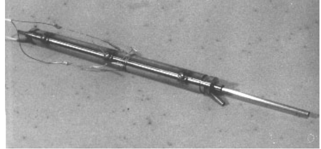
Figure 4: 30 cm-long superconducting undulator with period 10 mm and the axis field ~ 5 kG. Diameter of StSteel chamber is 6 mm, wall thickness 0.1mm.
