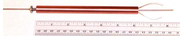
Figure 4: SC undulator model. Iron cylindrical shield for end trimming and ring jumper are visible here. One end of undulator has Copper jacket of ~12mm in diameter hides soft iron semi-cylinders having diameter ~9.8 mm.
