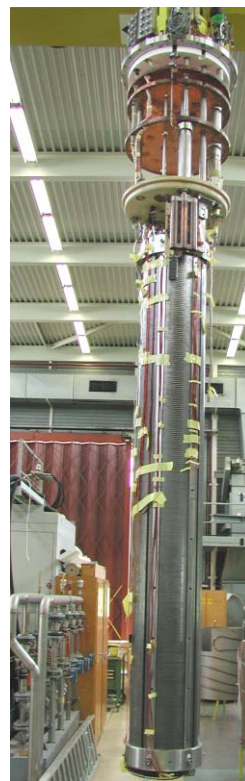
Fig. 1: Quadrupole suspended before being inserted into its vertical test cryostat.
