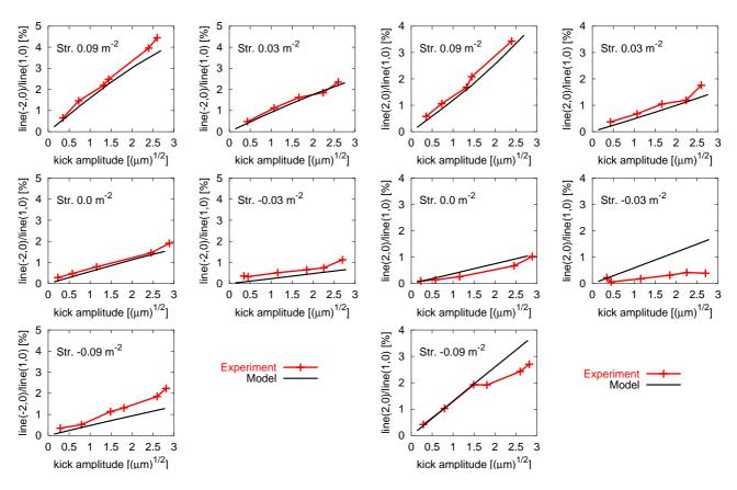
Figure 2: Measurement of the third order resonance. The normalised amplitude of the spectral line (-2,0) is plotted versus horizontal betatron amplitude for five different strengths of the sextupole. Experimental results are multiplied by the decoherence factor of 2 and predictions from the model are shown.
