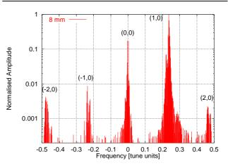
Figure 1: Fourier spectrum of the complex signal from pick-ups yo5-bh10 and yo5-bh12 for the unchanged RHIC and for an oscillation amplitude of 8 mm. The label (m,n) means that the frequency is equal to  $m\nu_x + n\nu_y$ .
