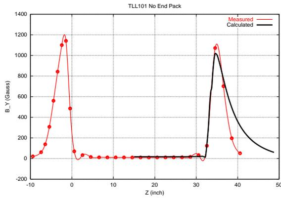
Figure 4: Measured transverse magnetic field in absence of endpicks. The integrated magnetic field is 240 G-m. The calculated field is also shown for comparison.
