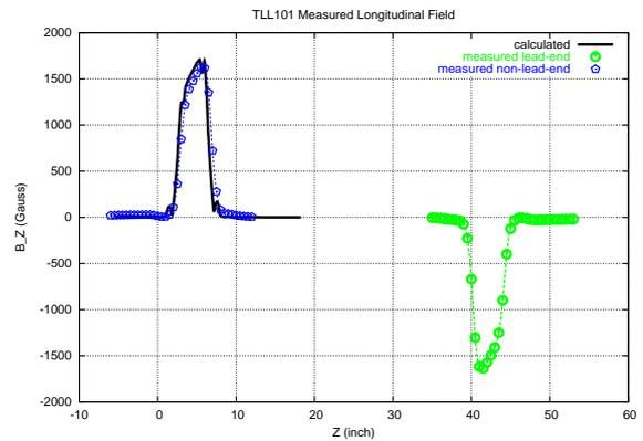
Figure 7: Measured longitudinal magnetic field in the field-free region. The calculated field is also shown for comparison.
