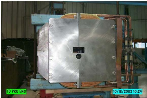
Figure 2: *Shield plate at the lead-end extremity.*
