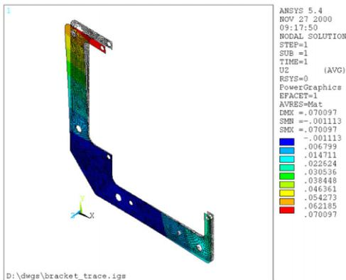
Fig. 5. Typical bracket deformed shape under maximum stress
