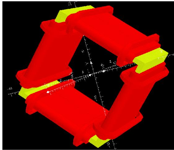
Figure 2. The windings of the dipole corrector.
