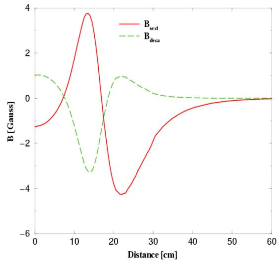
Figure 3: The calculated strength of the first two allowed multipoles ( $B_{sext}$ , and  $B_{deca}$ ), of the dipole corrector magnet, plotted as a function of the distance from the center of the magnet and along the beam direction.
