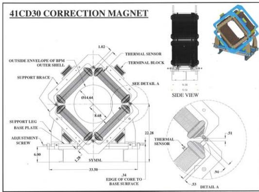
Fig. 4 Standard design of all corrector magnets
