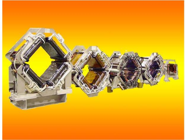
Figure 1. Actual picture of Corrector Magnets for SNS. (From left to right: 41CDM30, 36CDM30, 27CDM30, 27CD30, and 16CD20)
