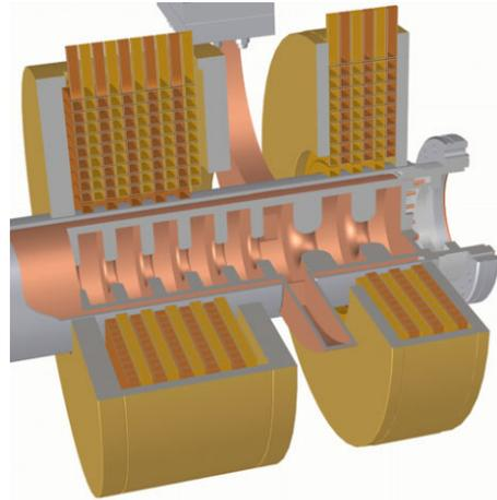
Figure 1: The first few cells of the hybrid photoinjector showing the emittance-compensating solenoid system.
