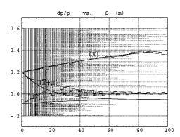
Figure 6: Average momentum of the  $\pi$ ,  $\mu$  and  $\pi + \mu$  beams as a function of their position along the decay channel, from Monte Carlo. Solid lines are theoretical, in the loss-free case [5].
