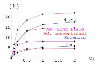
Figure 5: Efficiency of the AG channel versus longitudinal emittance  $\epsilon_l/\pi$  (eV.s) for values of transverse emittance  $\epsilon_{x,z}/\pi=1$  cm and 4 cm. The solenoid case is also shown for comparison.
