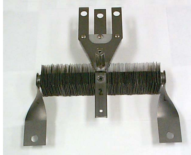
Figure 4 : ISAC fined target. It is the same target as shown in figure 2 onto which we have installed the fins.
