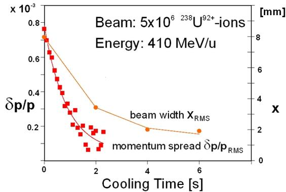
Figure 5: Results of stochastic cooling experiment at ESR (see text).
