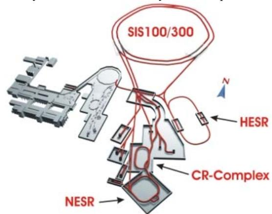
Figure 1: Preliminary layout of the proposed accelerator/storage ring facility at GSI (see text below).
