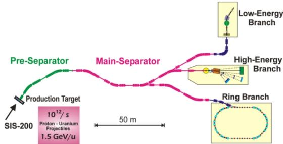
Figure 2: Layout of the Super-FRS [3], a magnetic separator equipped with super-ferric dipole and quadrupole magnets. The maximum bending power  $B \times \rho_{\max}$  is 20 Tm, the resolving power  $M/\Delta M$  about 1500.
