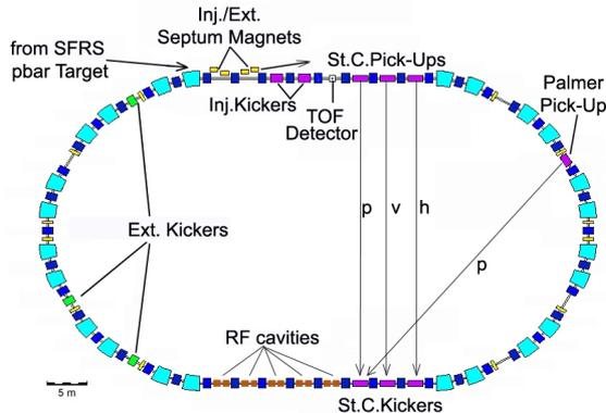
Figure 3: Layout of the Collector Ring CR. The ring will be equipped with superferric dipole magnets. The Palmer pickup is necessary only for rare isotope beams at the beginning of momentum cooling (too strong unwanted mixing).
