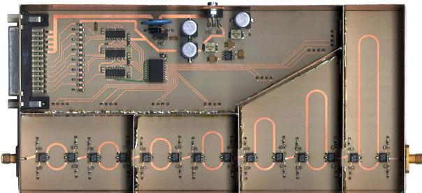
Figure 6: Prototype of a 1.27 ns-delay electronically switched in steps of 10 ps.
