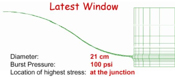
Figure 9: Improved absorber window design.
