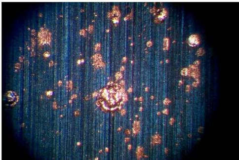
Figure 6: Be window surface showing sputtered copper.
