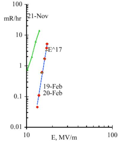
Figure 7: Background levels for copper windows (upper curve) and beryllium windows (lower curve) under identical magnetic field conditions.
