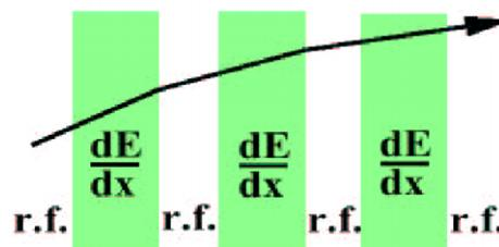
Figure 2: Schematic of ionization cooling process.
