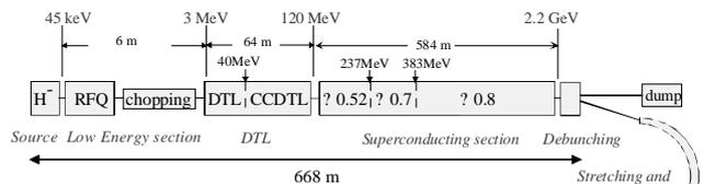
Figure 4: Diagram of proposed SPL configuration at CERN.
