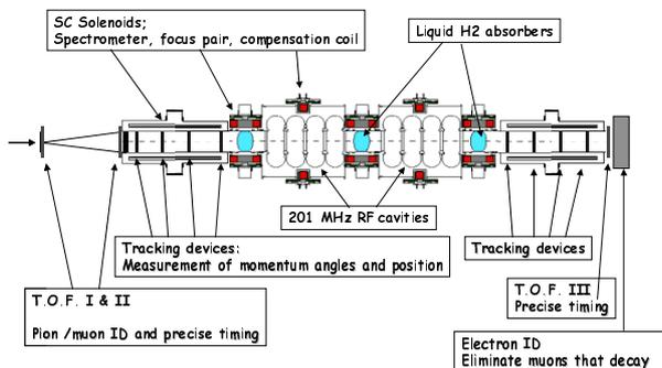
Figure 12: Schematic layout of MICE.
