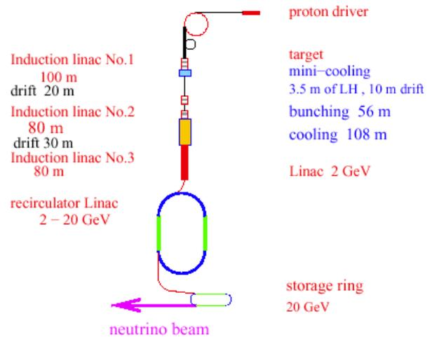
Figure 1: Schematic of Neutrino Factory layout, taken from Ref. [2].
