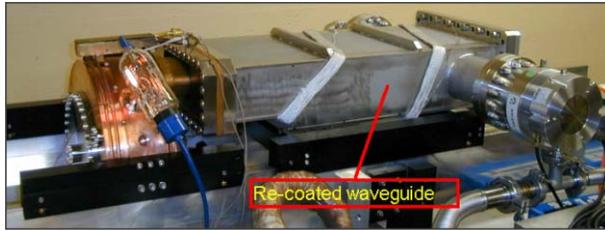
Figure 5: 805 MHz pillbox cavity used in high-power tests at Fermilab.
