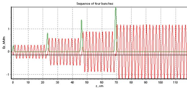
Figure 1. Single mode 13.625 GHz structure, 4 bunch (2-6-10-14) nC Ramped Bunch Train  $\omega_z = 0.4$  cm, Structure parameters are presented in Table 1.
