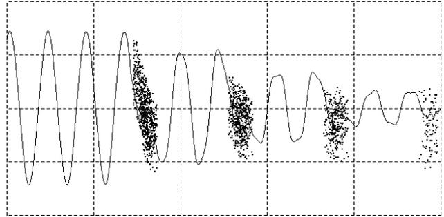
Figure 4. Beam dynamics simulations of the optimal (2-6-10-14) nC RBT, FODO focusing applied, 60 cm passed.
