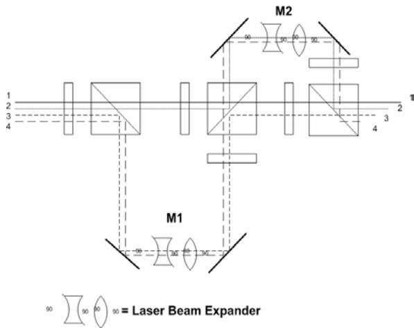
Figure 3. Adjustable and Variable Pulse Radius laser multisplitter design.
