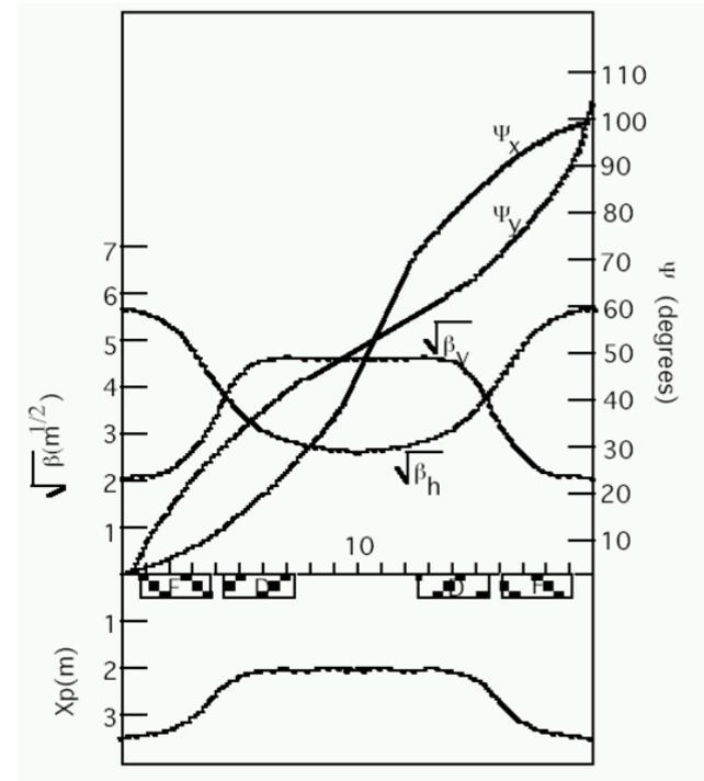
Figure 3: Booster lattice showing the correspondence between focusing and defocusing magnets and the horizontal and vertical beta functions. The vertical high  $\beta$  region is in the long straight section, while the horizontal high  $\beta$  region is in the short straight section [4].
