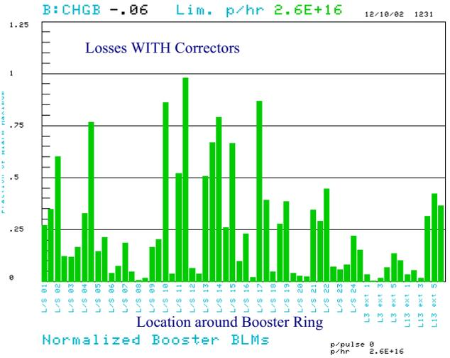
Figure 6: Normalized Booster losses as a function of position around the ring WITH ramped correctors to change the vertical beam position. Note that the losses around L/S 22 and 24 have been significantly reduced.
