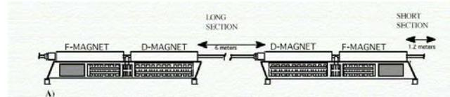
Figure 1: A Booster lattice cell [4], consisting of a focusing magnet, defocusing magnet, long drift, defocusing magnet, focusing magnet, and a short drift (FDOODFO).
