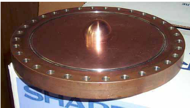
Figure 2. Twelve-inch-diameter Copper-plated stainless-steel Conflat disk and electrode.
