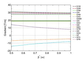
Figure 5: The gradient strengths for protons at 100 GeV vs.  $\beta^*.$
