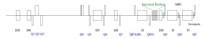
Figure 4: A schematic for half of the RHIC insertion. The quadrupoles Q4, Q5 and Q6 have associated trim quadrupoles. Q4 and Q5 trims are set to the same, but opposite strengths. Antisymmetry is broken for the trim quadrupole at Q6 and the quadrupoles at QFA(B). This leads to 12 adjustable parameters (including QF and QD).
