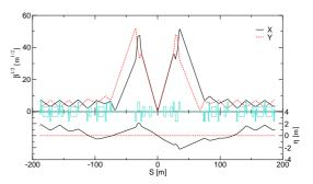
Figure 3: The RHIC insertion optics with  $\beta^* = 0.5m$ .
