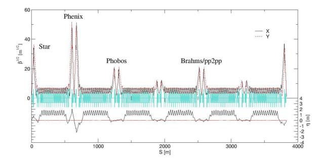
Figure 6: The RHIC optics parameters. The Star insertion is set to  $\beta^* = 1m$ , Phenix has  $\beta^* = 0.5m$ , Phobos and Brahms are at  $\beta^* = 3m$  and the remaining insertions have  $\beta^* = 10m$
