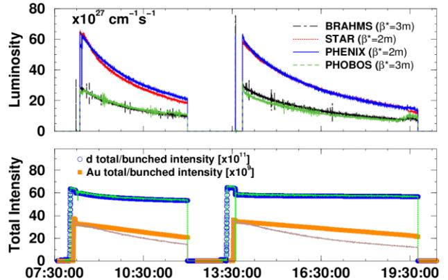
Figure 2: Two typical RHIC FY03 dAu stores, showing beam current ( $\times 10^{9/11}$  Au/p, total and bunched) and luminosity lifetime. Luminosity lifetime was dominated by gold beam lifetime and IBS-driven debunching and emittance growth. Time between stores was about 1 hour.
