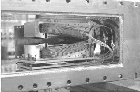
Figure 6: Picture of the massless septum magnet.
