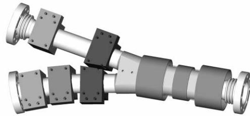
Figure 1: Injection Y assembly with magnets installed.
