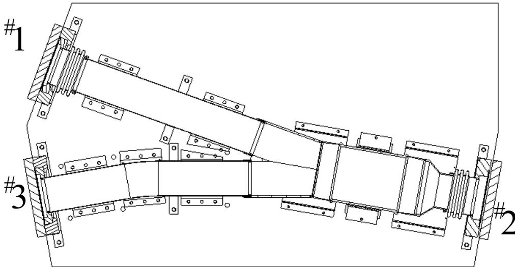
Figure 2: Cutaway view of injection Y assembly.
