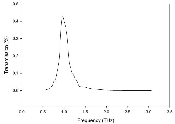
Figure 4: Terahertz band-pass filter.
