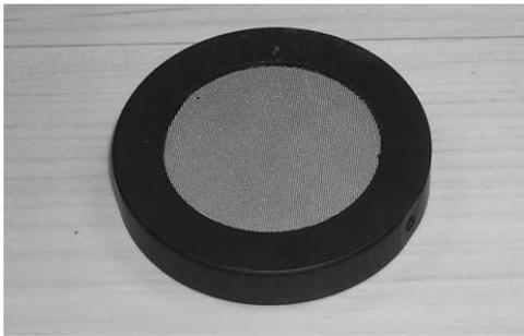
Figure 3: Etched steel terahertz filter.
