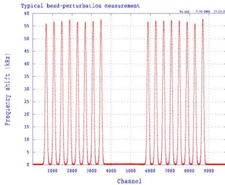
Figure 7. Bead pull measurement on hot-model cavity
