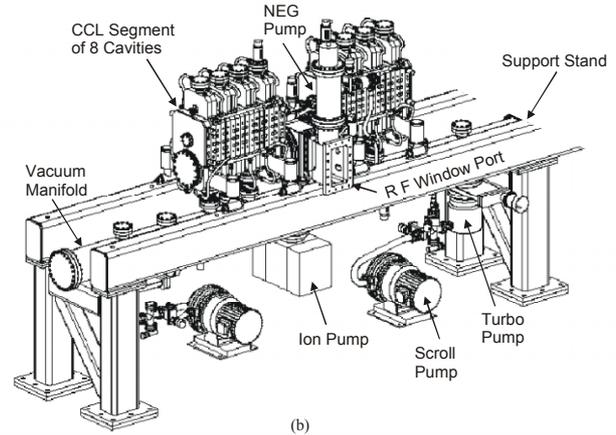
Figure 1. CCL hot model on support stand
