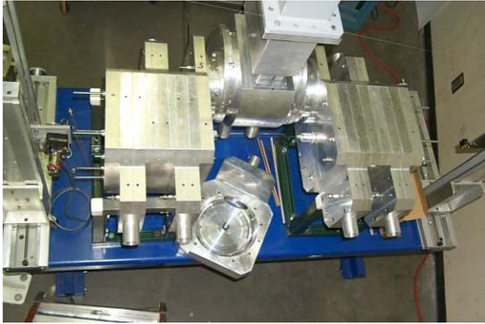
Figure 3. Example of cold model with bridge coupler
