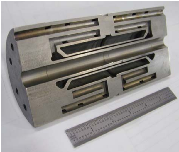
Fig. 4: Bonded Lens, before post-bond machining.
