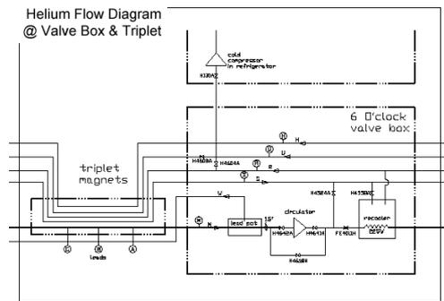
Figure 6: Schematic drawing of the RHIC cryo system. Helium pressure transducers are installed in the five transfer lines, namely the supply line (S), the return line (R), the utility line (U), the heat shield (H), and the magnet line (M). Only three of the six power leads at the quadrupole triplet cryostat are shown, labeled A, B, and C.
