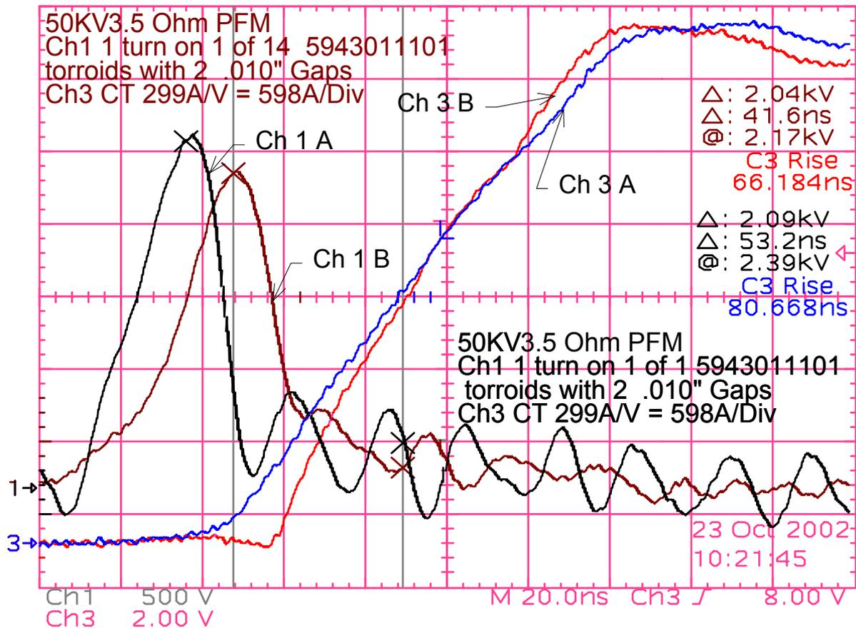
Figure 1 Scope trace from test stand. Ch 3 A is with only one toroid and Ch 3 B is with 14 toroids.
