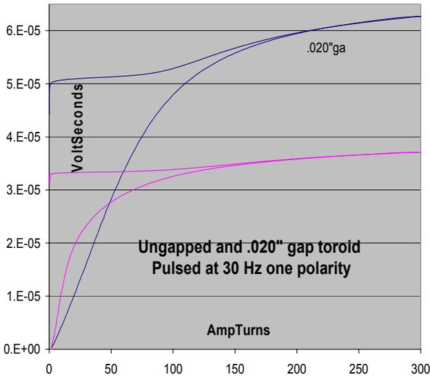
Figure 2 Measurements on 5943011101 toroid shows how many volt seconds can be applied before the toroid saturates.
