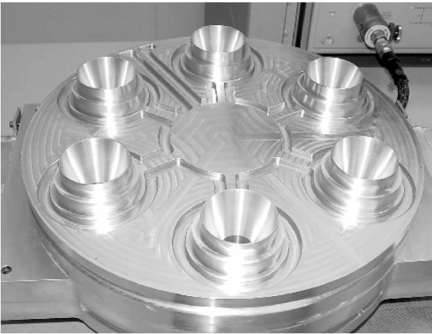
Figure 3. Aluminum output cavity model during rf cold testing.
