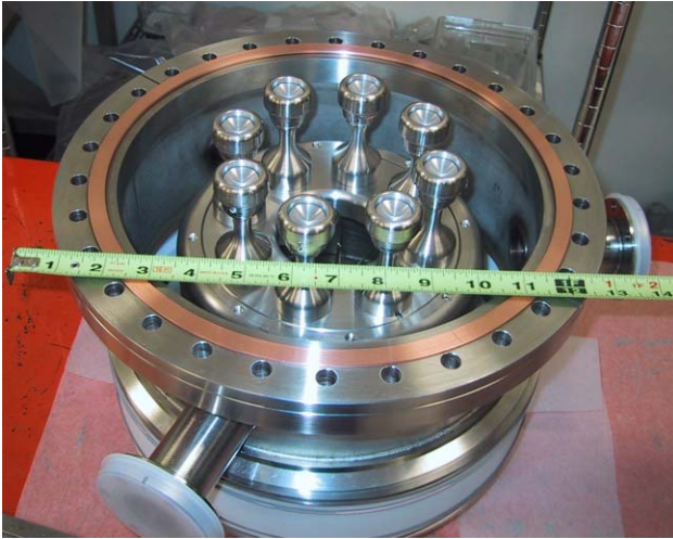
Figure 4. Eight beam, multiple beam gun under construction
