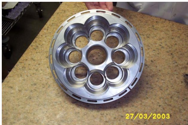
Figure 2. Field shaping iron in cathode-anode region
