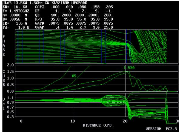
Figure 6: The JPNDISK simulation. Up to down: input parameters, Applegate plot, RF current verse z, velocity spread verse z.
