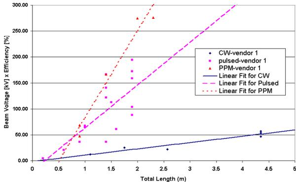
Figure 3: Beam voltage × efficiency vs. total length.
