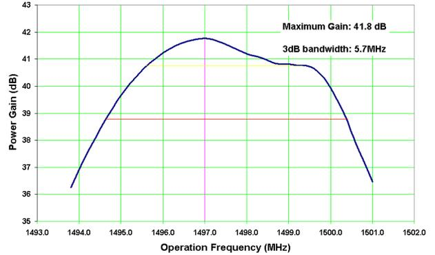
Figure 9: JPNDISK calculated gain and bandwidth.
