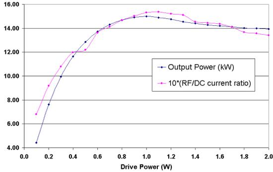
Figure 7: JPNDISK calculated output power verse input.
