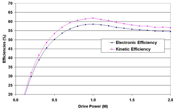
Figure 8: JPNDISK calculated efficiency vs drive power.
