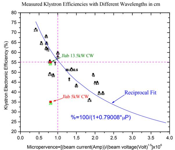
Figure 1: Klystron efficiency vs beam perveance.
