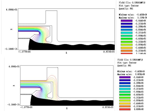
Figure 4: TRICOMP simulations in gun section. The potential at the cathode is  $-16kV$ ; at the mod-anode is  $0kV$  in top plot and  $-4kV$  in bottom plot.
