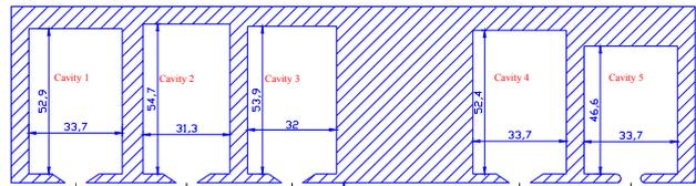
Figure 11: Klystron cavities designed by Superfish. All dimensions are in mm.
