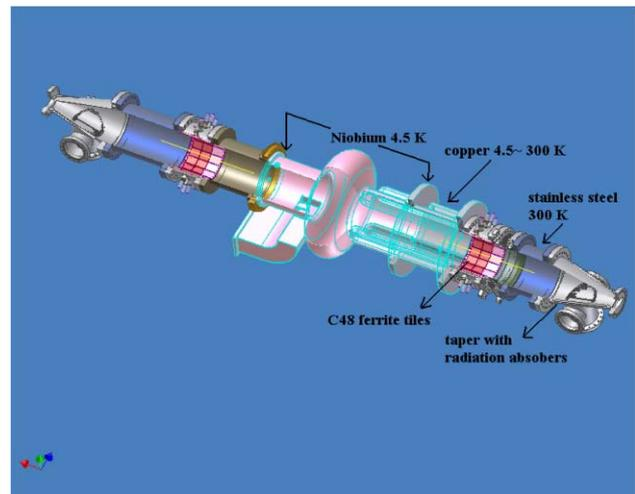
Figure 1: Layout of SC rf module used in the numerical simulations for the HOM studies at TLS. The taper design has been modified in order to fit into the vacuum chamber of storage ring at TLS.
