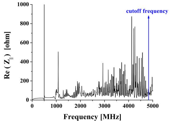
Figure 2: The real part of longitudinal impedance spectrum of SC rf module obtained from numerical simulations for TLS storage ring. The property of C48 ferrite tiles is set at a frequency of 4750 MHz.
