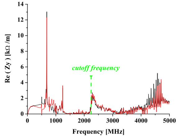
Figure 3: The vertical impedance spectrum calculated with vertical beam offset of 15 mm (black) and -15 mm (red) respectively. The lowest cutoff frequency of the transverse waveguide modes in the vertical direction is 2.237 GHz.
