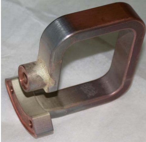
Figure 2. Buncher #2 coupling loop with a failed soldering joint.
