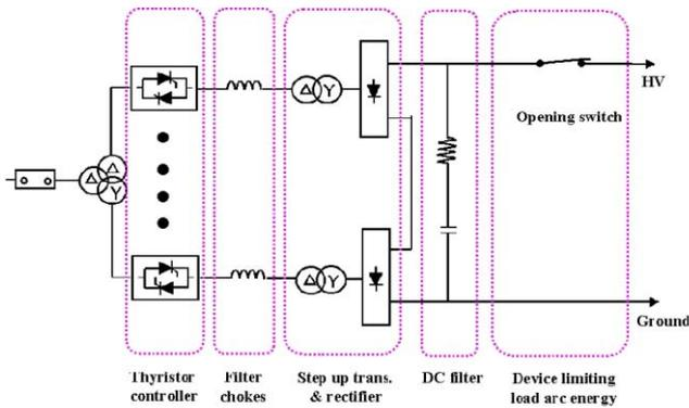
Figure 2 : Schematic of high voltage power supply
