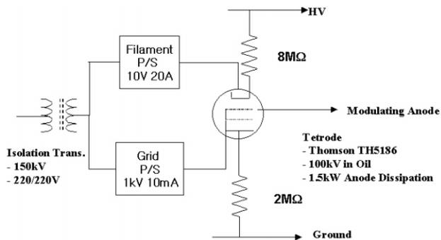
Figure 3 : Schematic of mod. anode power supply
