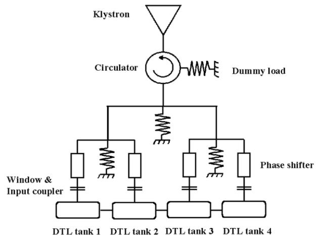
Figure 1: Schematic of RF power delivery system for 20MeV DTL
