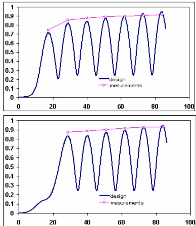
Fig.3: The designed and measured amplitude of electric field distribution for FXB “fat lip” (upper) and waveguide (lower) couplers
