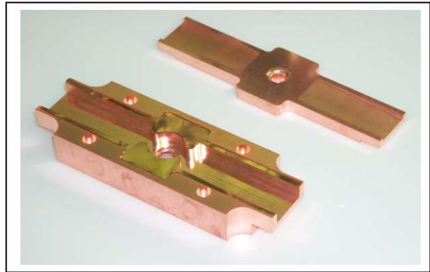
Fig. 7: “Fat lip” input coupler main body and plate.
