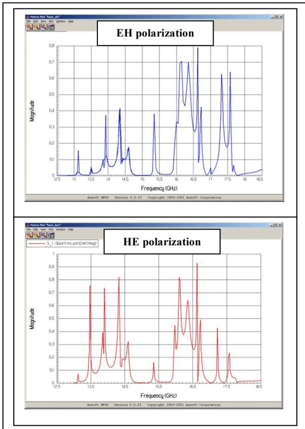
Fig. 6: HOM's spectrums for FXC structure.
