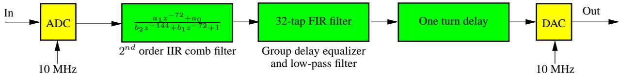
Figure 5: A block diagram of one channel of PEP-II double-peaked comb filter
