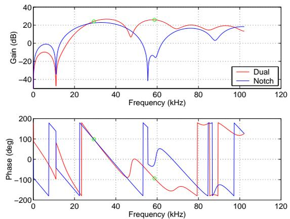
Figure 4: Magnitude (top) and phase (bottom) responses of a dual-peak and peak-notch filters used in control and study of quadrupole instabilities in DAΦNE  $e^-$  ring
