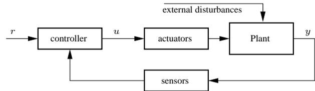
Figure 1: Generalized block diagram of a feedback system
