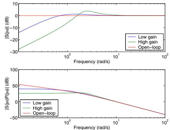
Figure 2:  $|S(j\omega)|$  for two loop gain settings as well as open-loop is shown on the top plot, while the gain from the input to the output of the plant is illustrated on the bottom.
