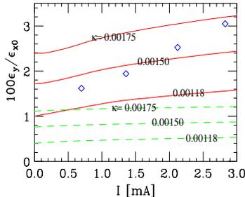
Figure 2: Comparison with ATF measurements. ( $\kappa$  in  $m^{-2}$ )
