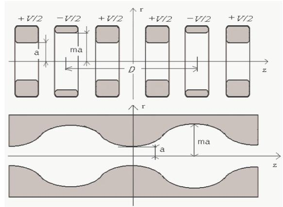
Figure 1: ARF and RFQ channels.
