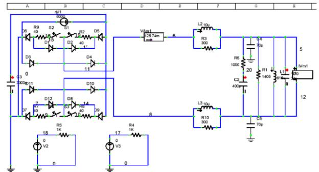
Figure 4: SPICE model of the circuit for the barrier RF power supply.
