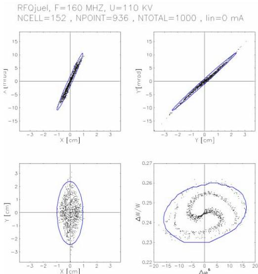
Figure 8: Beam distribution after the matching section.
