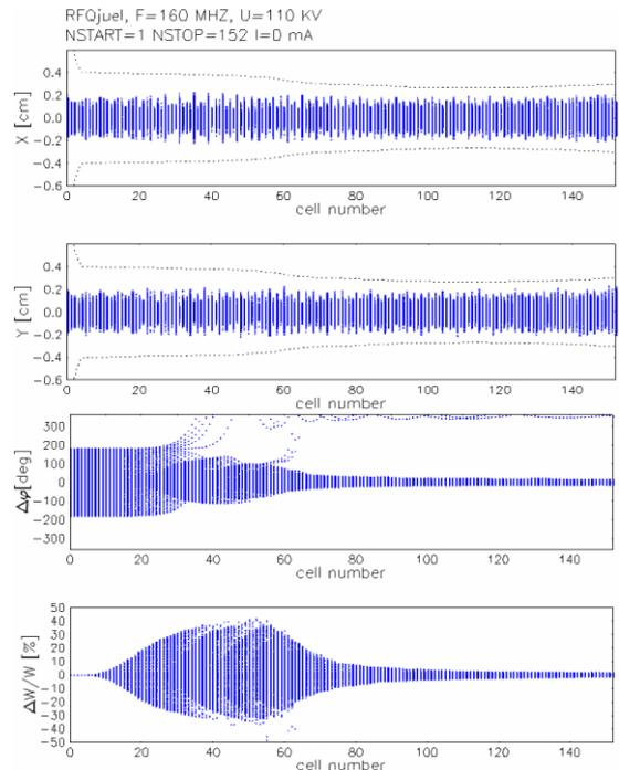
Figure 5: PARMTEQ simulation of the RFQ. The upper two graphs display the transverse beam envelope. The longitudinal evolution of the beam is shown in graphs three and four.
