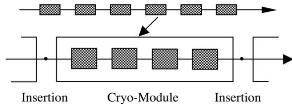
Figure 2. Configuration of a Proton Super-Conducting Linear Accelerator
