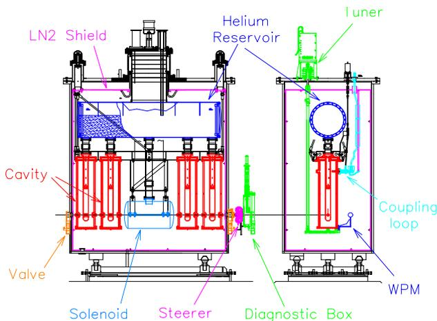
Figure 5: The ISAC-II prototype medium beta cryomodule.
