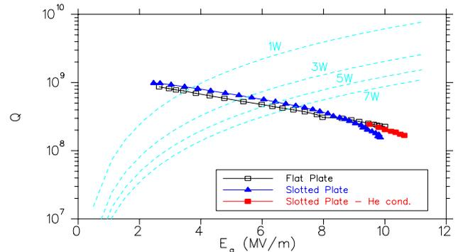
Figure 4: RF cold test results comparing cavity performance with a flat tuner plate and the new slotted plate.
