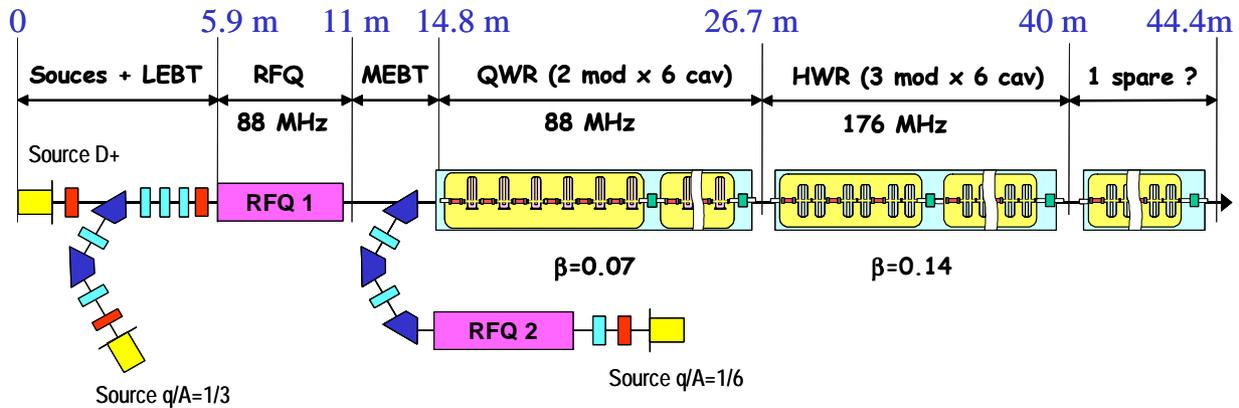
**Figure 1 : Architecture of the SPIRAL 2 Linac**
