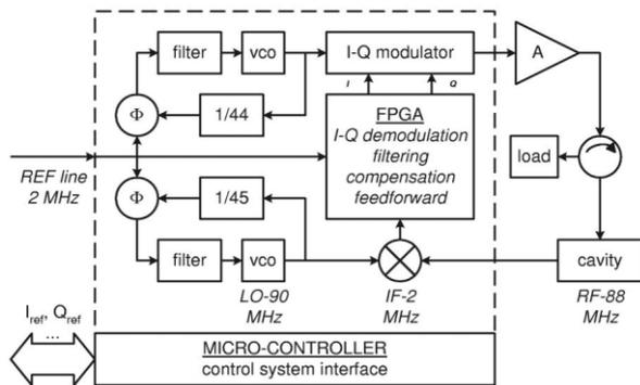
Figure 4 : Block diagram of the LLRF system.
