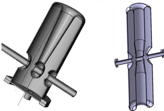
Figure 3 : QWR and HWR geometries
