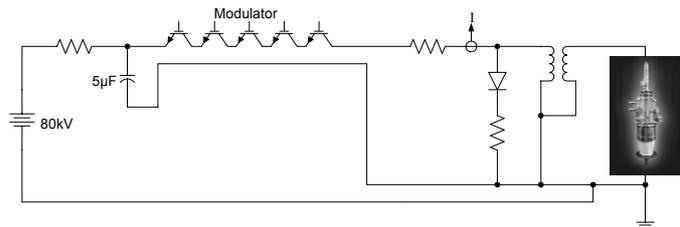
Figure 1: NLC Hybrid modulator schematic. The solid state switch pulses 3500 A at 80 kV to drive two 500 kV 265 A klystrons.
