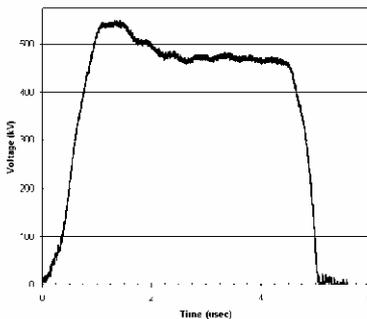
Figure 4: Fast pulse data at 500 kV, into a 990Ω load.
