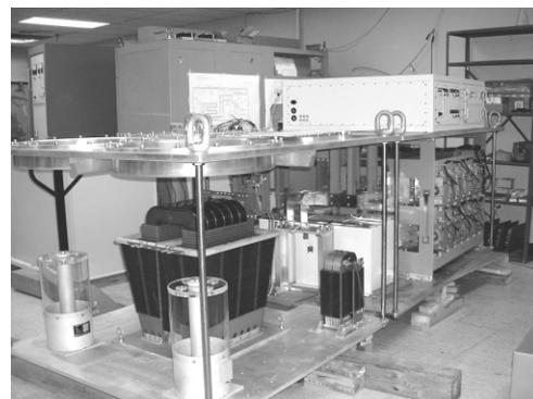
Figure 2: Hybrid modulator assembly, ready for immersion in oil.
