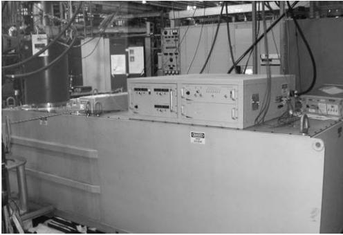
Figure 3: Hybrid Modulator in tank at SLAC, with a SLAC 5045 klystron in a load socket.
