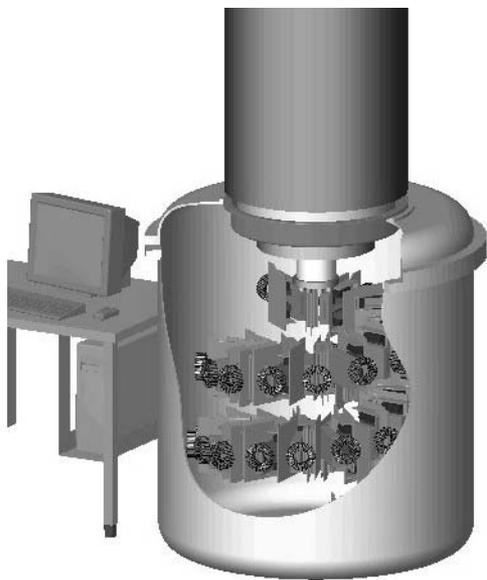
Figure 8: Proposed 500 kV “desk size” 250 A modulator.
