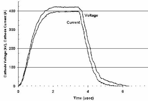
Figure 5: Hybrid modulator operation at SLAC. Load is 5045 klystron, with the cathode operated in temperature limited mode for an effective 1.5 μP load.
