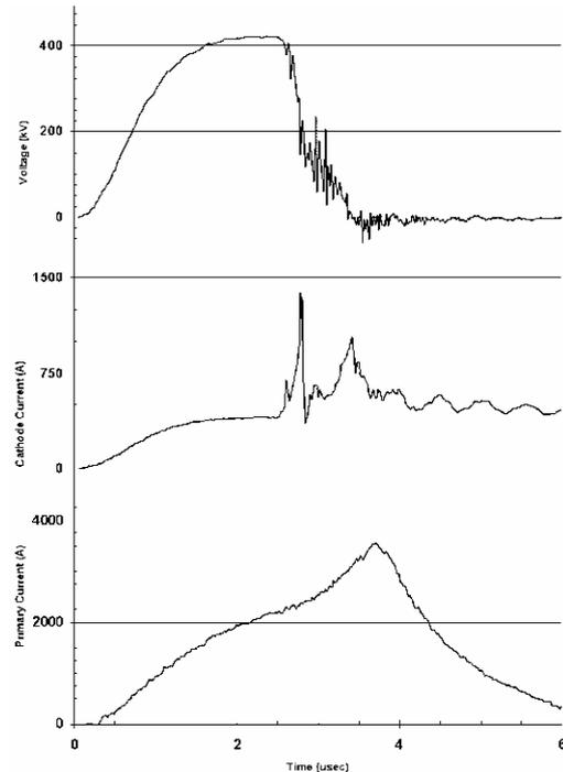
Figure 6: Hybrid modulator with a load arc at 420 kV. The load (5045 klystron) arcs at about 2.5 μs. The switch safely opens under full *fault* primary currents. The lag time is about 1 μs between arc occurrence and switch opening. (Primary current shown at reduced bandwidth.)
