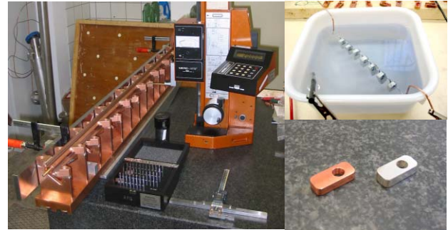
Figure 4: Adjustment of the electrodes outside of the tank on the left. Electrolytic process of silver plating and plated distant plates on the right.
