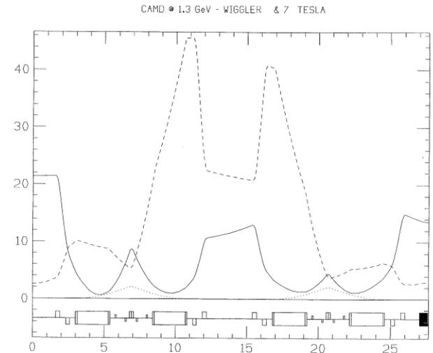
Figure 2 Optical functions for half ring with the focusing effect of the wiggler uncorrected. Black spot in the right is the wiggler location.
