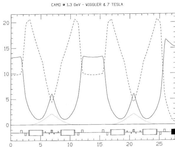
Figure 4. Low beta with zero  $\eta$ -function
