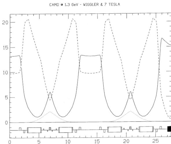
Figure 4. Low beta with zero  $\eta$ -function
