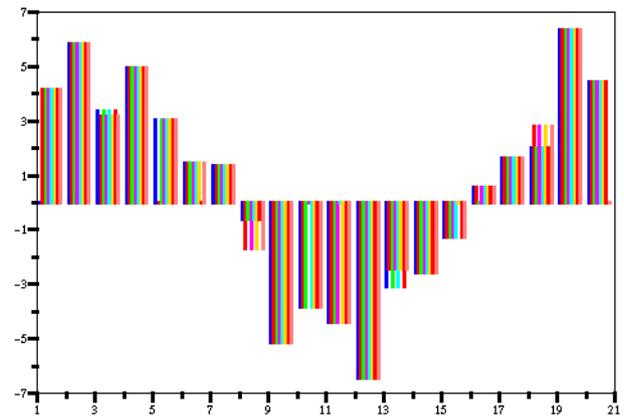
Figure 6 Theoretical response matrix for the standard lattice. 20 PUE reading organized in coloured 8 trims families
