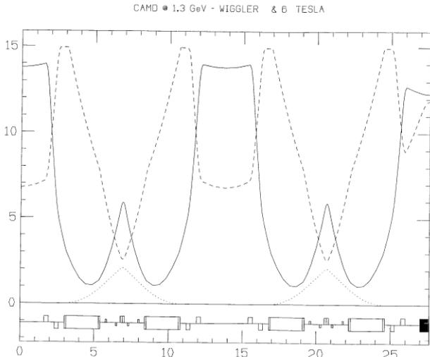
Figure 3 Shunted configuration. Vertical beta function increases in the wiggler straight
