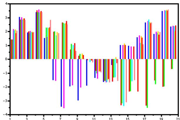
Figure 10 Measured response matrix of non zero dispersion function low beta configuration with the wiggler at 7 Tesla.
