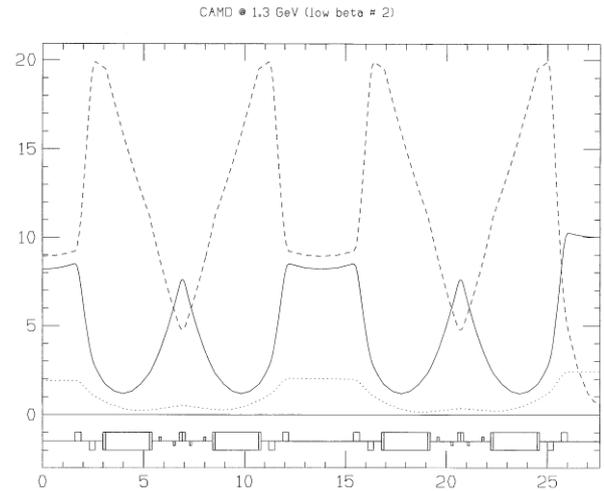
Figure 5. Low beta configuration with non zero  $\eta$ -function. No wiggler field in this plot
