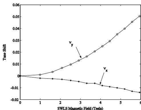
Figure 4: The measured tune shifts of SWLS.
