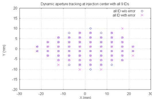
Figure 2: Dynamic aperture simulated from PATPET with field errors and all insertion devices.
