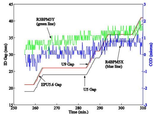
Figure 3: With the follow-gap look-up table and global orbit feedback system, the orbit drift of the field scan of U5, U9 and EPU5.6 can be reduced from a few hundred microns to a few microns. When the gaps of U5, U9 and EPU5.6 are scanned from 19, 21, and 21 mm to 39, 41, and 41 mm, the closed orbit distortions indicated by the R4BPM5X (blue) and R3BPM3Y (green), those are used in the faster orbit feedback system, are within 2 microns in both horizontal and vertical planes.
